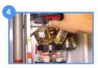
Spin the hand wheel to the right to lower the manifold.
