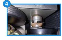
If the plastic motor coupler does not line up with the upper hub, use the hand wheel to put it into place.
