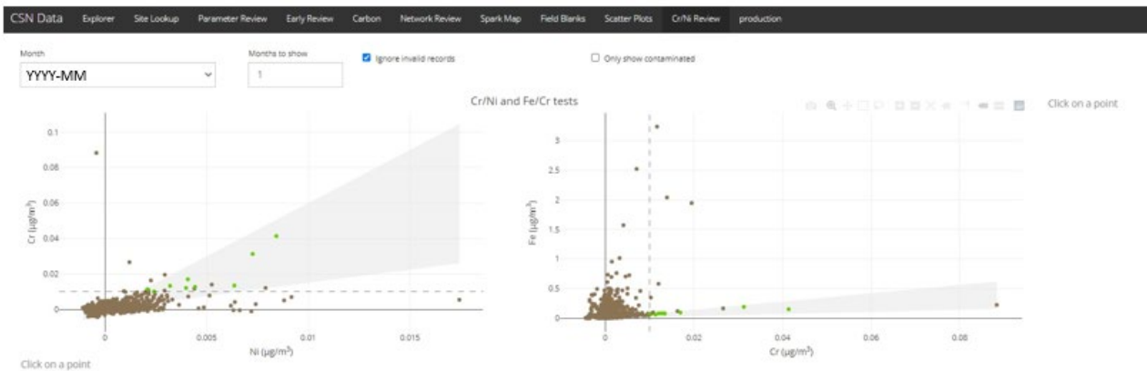
Figure 11. The Cr/Ni Review tab of the CSN Data web app visualizes the two ratio tests used in the Chromium/Nickel contamination criteria with a line at the limiting Chromium concentration. Filters meeting the criteria are highlighted in green. Clicking on a point will display a time series of the three species used in the criteria.
