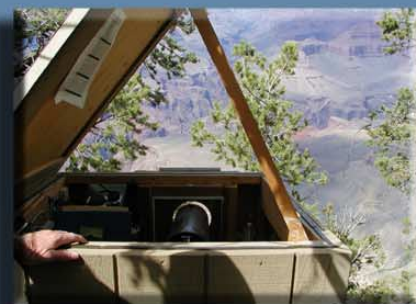
Located near the Yavapai Museum, the IMPROVE transmissometer measures air quality between the rim and the receiver station at Phantom Ranch in the inner canyon.
