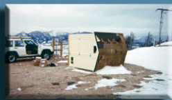
Winds blew the shelter on its side before the crew arrived to install the aerosol sampler.
