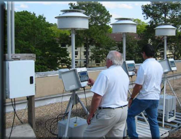
Collocated samplers at NAREL used to make replicate filter samples.
