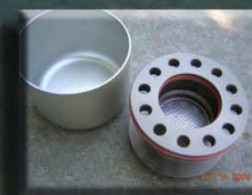
A new inlet design was easier to clean but still clogged occasionally.
