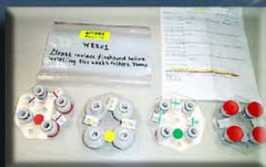
Four filter cartridges: Red for Module A Yellow for Module B Green for Module C Blue for Module D
