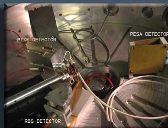
Figure 1: ORTEC 2800 series scattering chamber with RBS, proton elastic scattering analysis (PESA), and XRF detectors
