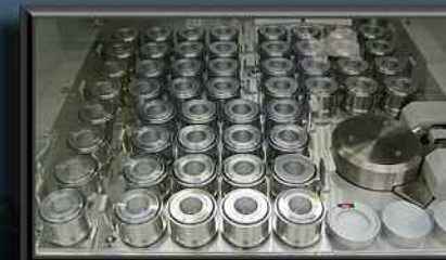
Epsilon 5 XRF filter analysis cups
