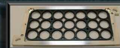
Epsilon 5 XRF filter analysis cups
