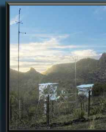
RAWS weather station under fire wraps
