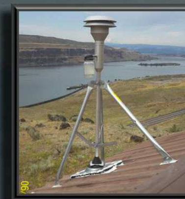
Tripod stabilizes the stack.
