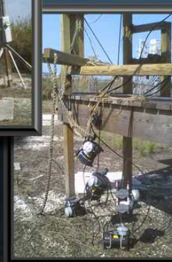
Breton Island (BRIS1), 2010: Hurricane Isaac left a lot of damage and nine feet of water in the area. Water had also gotten into the meter box.
