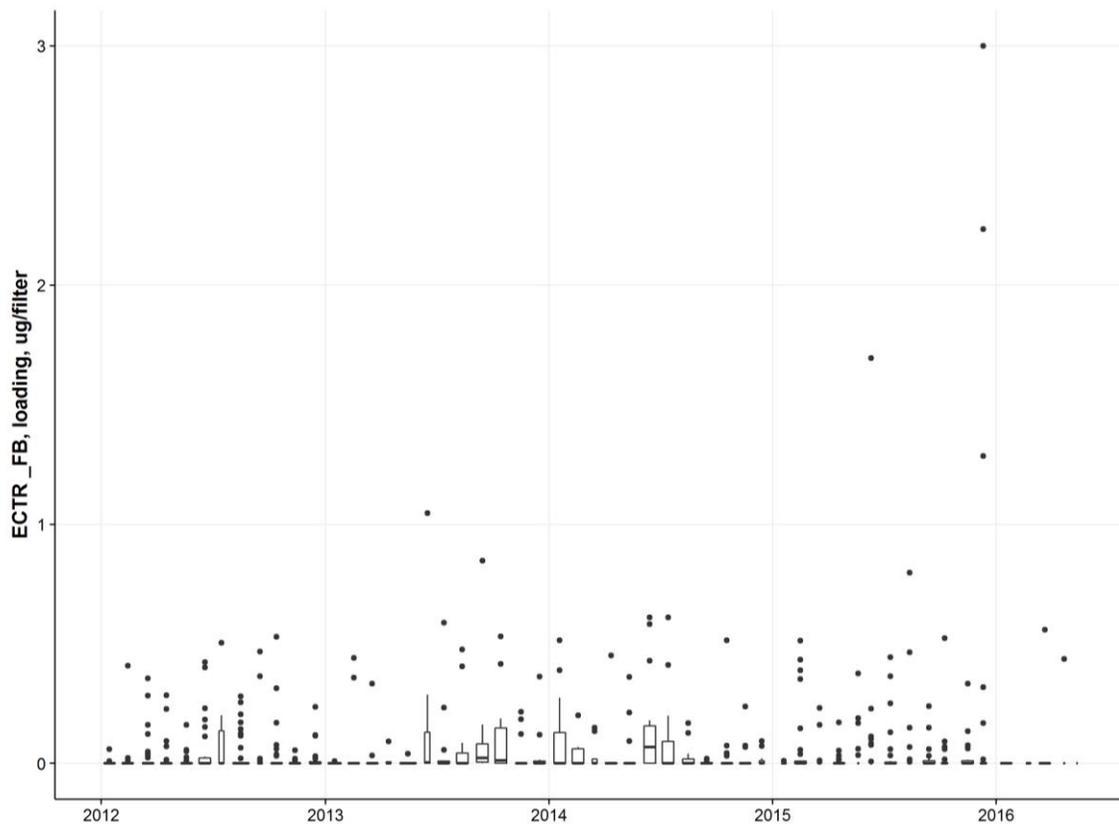
**Figure 17:** Time series of organic carbon artifact on quartz filter field blanks.
