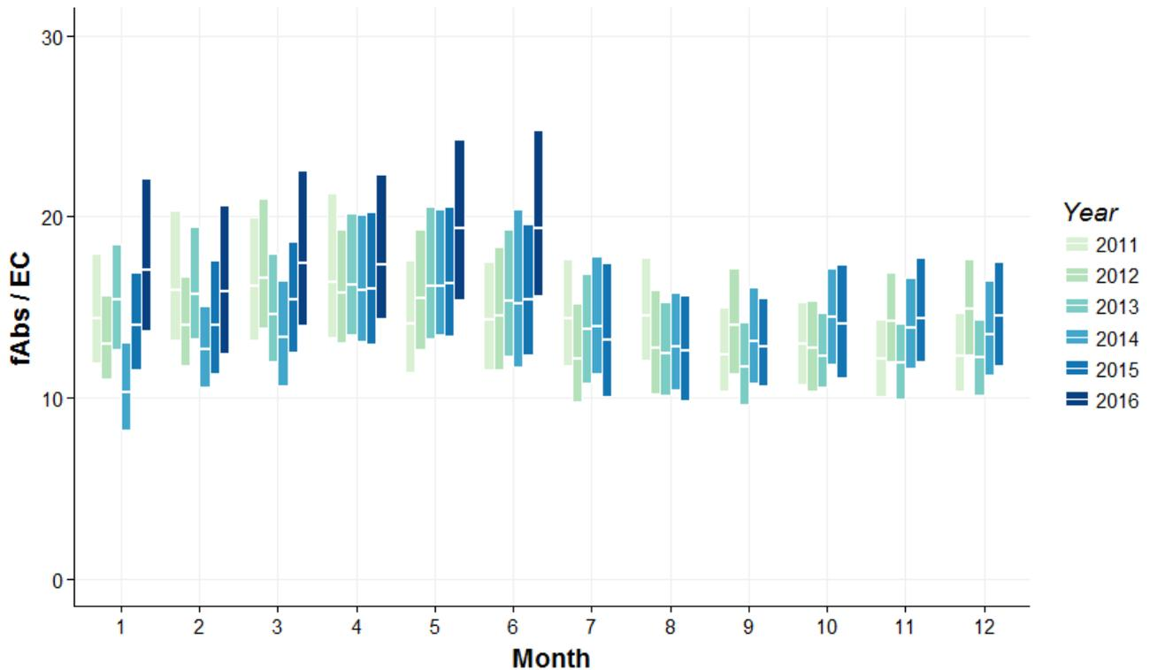
Higher Fabs/EC ratios are observed in early 2016 (January through June), corresponding with lower EC concentrations (Figure 4). This shift in the ratio coincides with the change in instrumentation discussed in Section 2.1.
