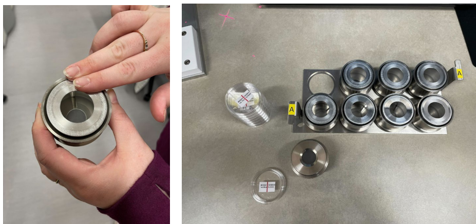
Figure 8. Sample holder cup handling and positioning.
