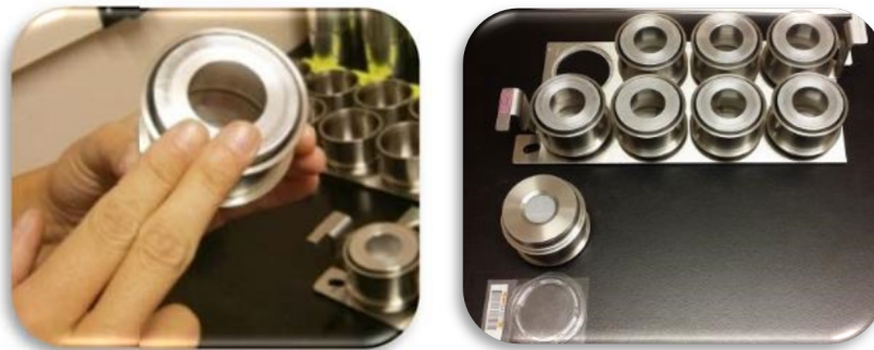
Figure 8. Sample holder cup handling and positioning.
