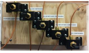
3. Turn the gas line valve to the "Closed" position (pointing down) for the gas to be changed.
