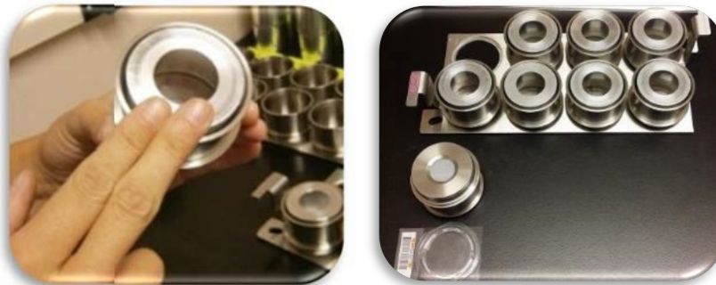
Figure 8. Sample holder cup handling and positioning.
