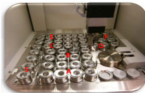
Figure 2. Sample changer compartment with trays.
